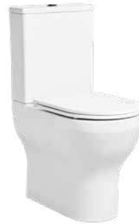
Comfort Height Fully Enclosed Close Coupled WC Spigot distance from wall 125mm 365(w) x 905(h) x 620(d)mm
